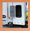
Side Access Doors Large 7" x 18" tall side doors can be added on either side
